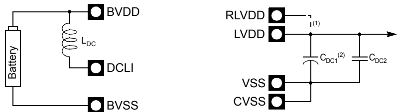
Figure 135. Battery DC-DC Connection
